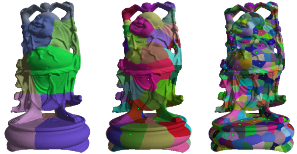
Fig. 2 Example of the results of k -means clustering ( k = 8 ) for the first three passes of the algorithm using five k -means iterations. Triangles belonging to different clusters are shown in different colors. Cluster representatives are shown as axis aligned boxes in green.
