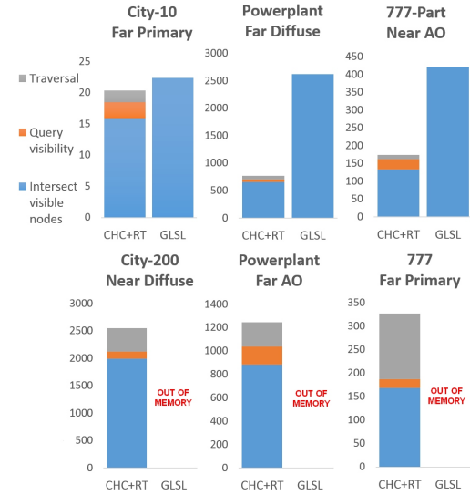
Figure 8: Traversal-time comparison of CHC+RT with GLSL split into the different phases of the algorithm.
