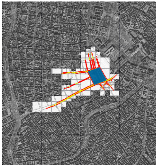
Figure 1.1: Offline visibility culling. The figure depicts 8\text{km}^2 of Vienna and a view cell of 0.1\text{km}^2 (shown in blue). The red objects form the PVS for the view cell.
