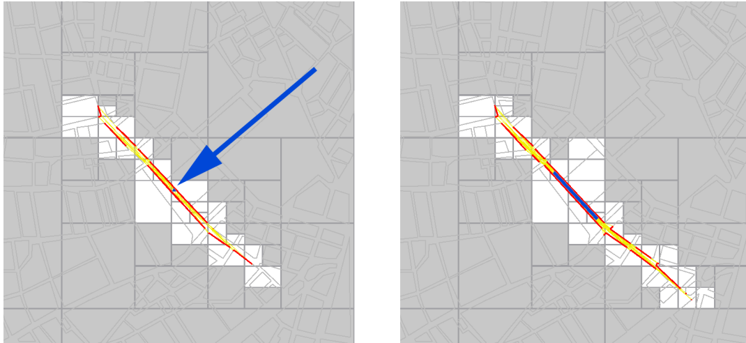
Figure 7.11: (left) A small view cell and its PVS. (right) The PVS for a larger view cell can be very similar.
