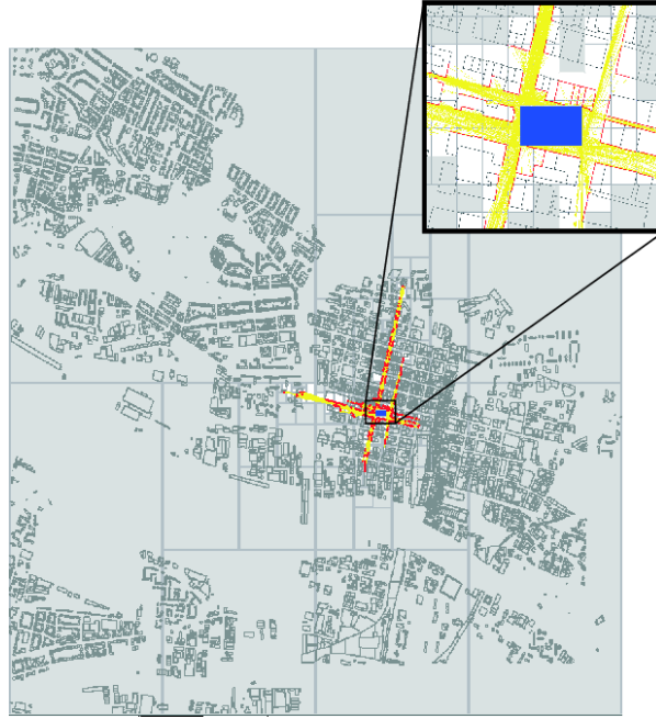
Figure 6.1: Illustration of the from-region visibility in 2D. The scene represents 25\text{km}^2 of Glasgow city. The 2D projection of the scene contains 94460 line segments. Parts of occluders visible from the given region are shown in red. Yellow line segments depict extremal lines that correspond to changes in visibility. Visibility computation took 700ms.
