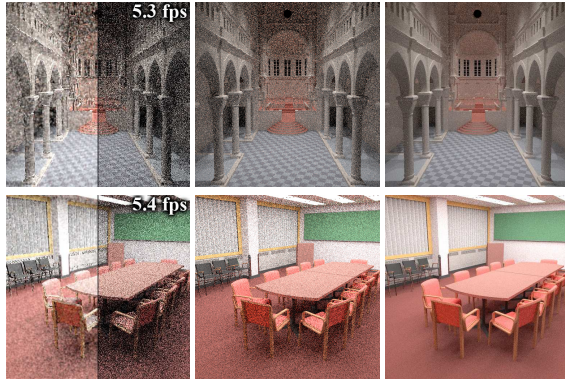
Figure 4: Interactive rendering of the Sibenik Cathedral and Conference Room. Each triple contains a filtered/original preview image with corresponding frame rates, and rendering results after 1 and 10 seconds of progressive refinement.
