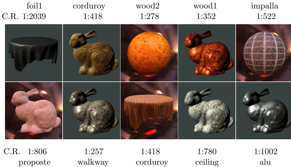
Figure 1: Example images rendered by the proposed BTF compression methods for illumination by point light and by different environment maps.
