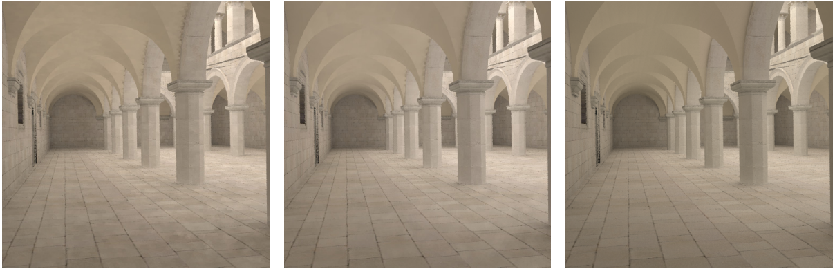
Figure 4.7: Cached irradiance interpolation using one screen pass (left), two passes (middle), and the reference image (right).
