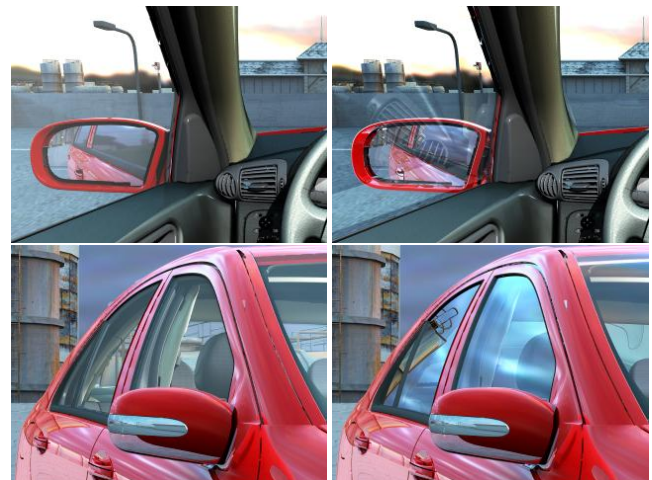
Figure 4: Realistic simulation of glass effects has a strong impact on the level of realism of a rendered image. Left: Rendering glass materials as semi-transparent surfaces as usually done in rasterization-based VR systems. Right: With a physically-correct, ray traced glass shader. Top: View from drivers seat (effect slightly emphasized to reproduce on paper). Note the reflection of the car interior over the left rear-view mirror. Bottom: View from the outside.
