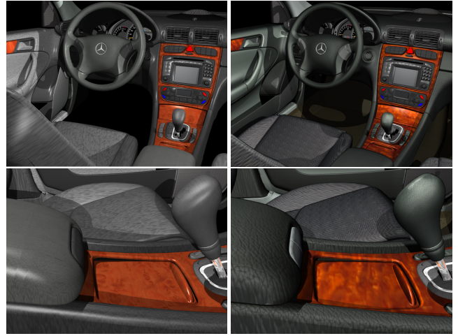
Figure 7: Comparison of using BTFs vs. the usual textured Phong surfaces by a view into the car's cockpit. Left: Textured Phong. Right: Using measured BTFs. Top: Entire cockpit. Bottom: Zoom onto the wood and leather.
