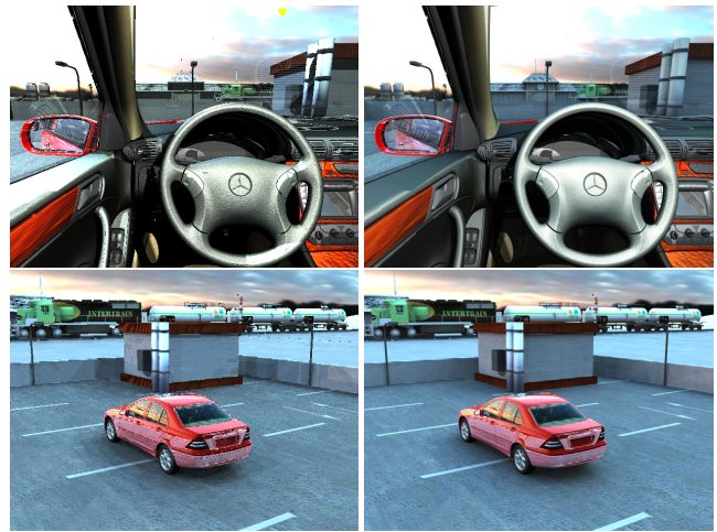
Figure 8: The final system. Top: Driver’s view of the interior. Bottom: Outside view. Note the smooth shadows, the correct reflections in the car’s paint, the subtle glass effects in the windshield, as well as the detailed interior. These views can be ray traced at 1.5 (top row), and more than 10 frames per second (bottom row) at 640 \times 480 pixels, respectively. Left: During camera motion. Right: After accumulating several frames.
