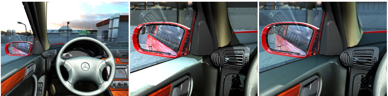
Figure 12: (a) Reflections of the interior in the windshield and side windows, when evaluating effects like glare, occlusion, or distraction (effects artificially emphasized to reproduce on paper). (b) Zoom onto the mirror, during interaction. (c) After accumulating several frames.
