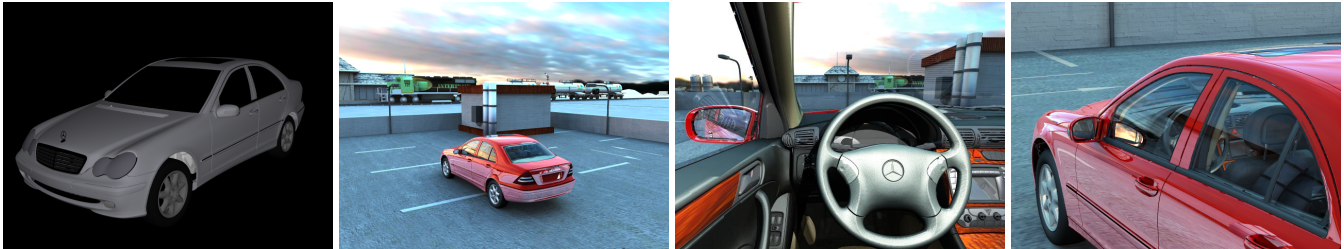
Figure 1: Several example screenshots from the presented framework, demonstrated on a complex Mercedes C-Class model: (a) The model consists of 320,000 Bézier patches and thousands of trimming curves that are directly and interactively ray traced without triangulation. (b) The model with ray traced shaders, e.g. glass and car paint, put into a surrounding scene made up of 200,000 triangles and a captured high dynamic range environment map. Note the accurate reflections, the refraction through the glass, and the smooth shadows from environment lighting. (c) The realistic interior appearance is achieved via a shader supporting bidirectional texture functions of measured samples from the corresponding real-world materials. (d) All these effects work together seamlessly, as can be seen on this view through the side window. At slightly reduced quality during interaction, these views can be rendered at 20, 14, 1.5, and 4.8 frames per second, respectively (640 × 480 pixels).
