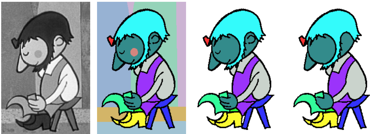
Figure 3.1: Different precision of segmentation: (from left to right) grey-scale image, nearly ideal segmentation, contour based segmentation, real regions with different color index.
