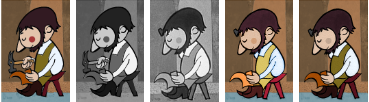
Figure 4.2: HSB vs. RGBI model: (from left to right) image with example colors, only luminance of example colors, original grey-scale image, color luminance modulation using HSB model and RGBI model.
