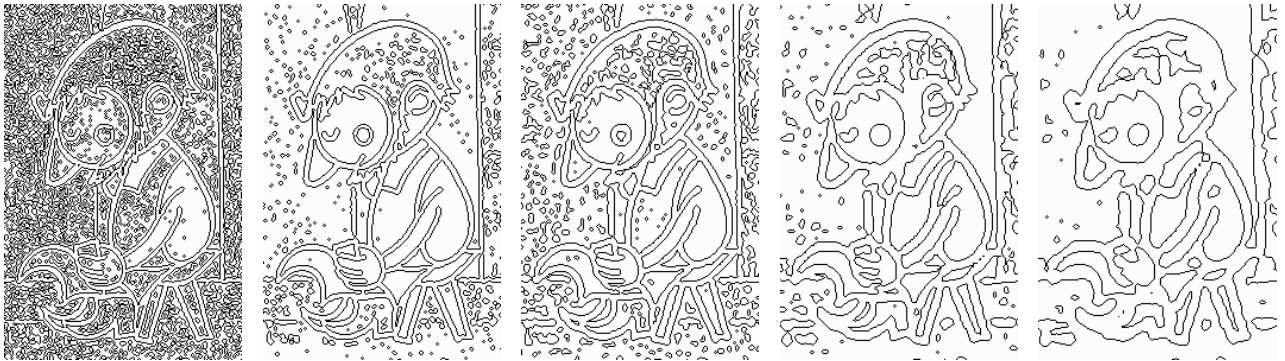
Figure 3.10: Scale-space of the L \circ G filter: (from left to right) \sigma = 1.0, 1.5, 2.0, 3.0, 4.0 .
