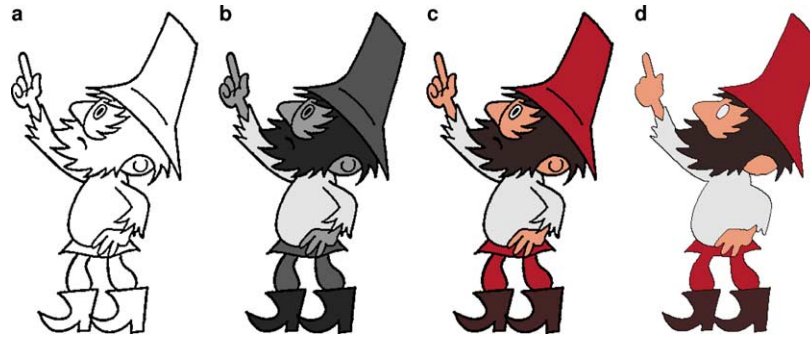
Fig. 4. Unsupervised segmentation in progress: (a) outlines, (b) regions, (c) color-to-region assignment, and (d) region growing.
