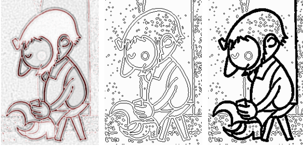
Figure 4: Contour detector in progress: approximation of the second-order derivatives (left), zero crossing (middle), flood-fill (right).
