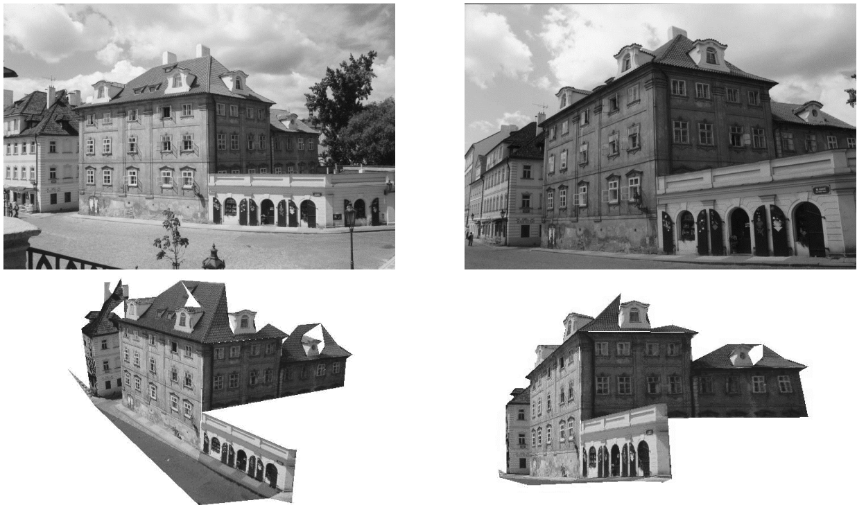
Figure 3: A 3D model of a single building, semi-automatically reconstructed from 7 photographs. Two input photographs and two shots of the output VRML model are shown. Notice that parts invisible on input photographs have not been reconstructed in 3D. (Courtesy of Center for Machine Perception, CTU in Prague)
