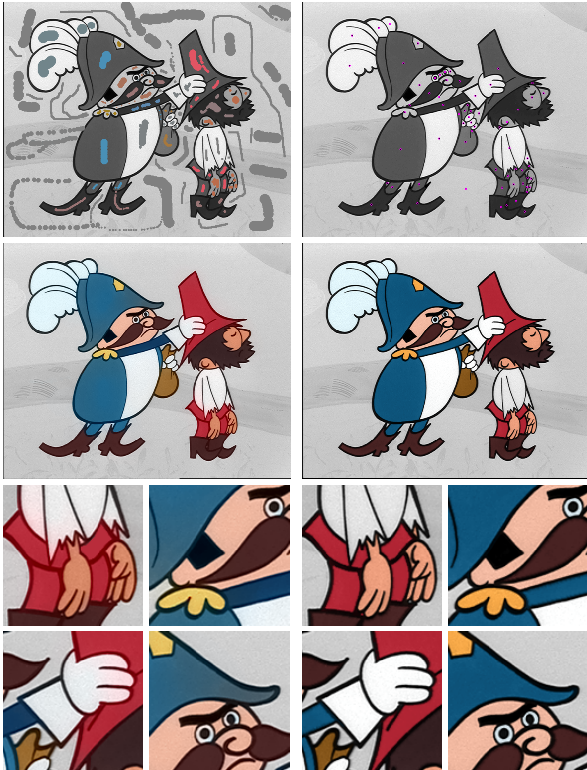
Figure 3.21: Experiments – visual quality comparison: colorization produced by Levin's framework (left) in contrast to the proposed approach (right): color markers (top), foreground layer colorization (middle), detail views (bottom).
